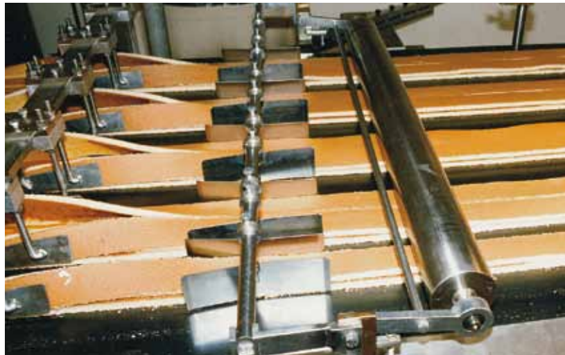
A Sandvik carbon steel belt provides the perfect base for finishing operations for sponge cakes, such as cutting, folding, layering, creaming, jamming and decorating.
